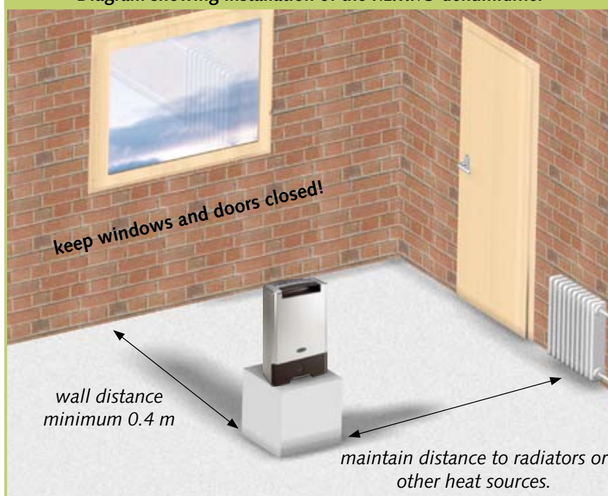
Diagram showing installation of the REMKO dehumidifier
